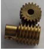
Worm gear - lots of torque but slow N:1 ratio (N = # teeth on spur gear)
